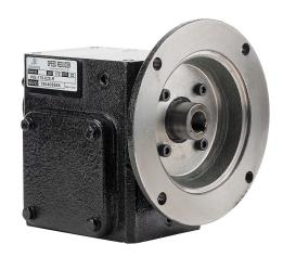
IronHorse heavy-duty worm gearbox, 20:1 ratio, 56C-Face input, right hand, 0.875in diameter output shaft, nominal 0.75hp at 1.0 SF, 737 lb-in mechanical output torque, 1-3/4in center distance, cast iron housing, tapped-base mount.
