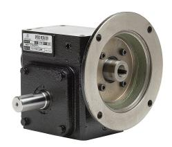
IronHorse heavy-duty worm gearbox, 20:1 ratio, 56C-Face input, left hand, 0.875in diameter output shaft, nominal 0.75hp at 1.0 SF, 737 lb-in mechanical output torque, 1-3/4in center distance, cast iron housing, tapped-base mount.
