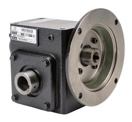
IronHorse heavy-duty worm gearbox, 20:1 ratio, 56C-Face input, hollow, 1in diameter output shaft, nominal 0.75hp at 1.0 SF, 737 lb-in mechanical output torque, 1-3/4in center distance, cast iron housing, tapped-base mount.
