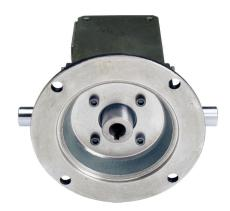
IronHorse heavy-duty worm gearbox, 20:1 ratio, 56C-Face input, dual, 0.875in diameter output shaft, nominal 0.75hp at 1.0 SF, 737 lb-in mechanical output torque, 1-3/4in center distance, cast iron housing, tapped-base mount.
