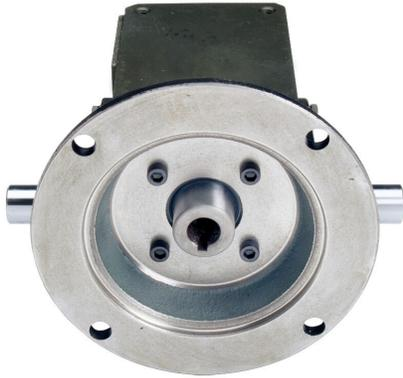
IronHorse heavy-duty worm gearbox, 20:1 ratio, 56C-Face input, dual, 0.875in diameter output shaft, nominal 0.75hp at 1.0 SF, 737 lb-in mechanical output torque, 1-3/4in center distance, cast iron housing, tapped-base mount.
