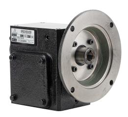
IronHorse heavy-duty worm gearbox, 15:1 ratio, 56C-Face input, right hand, 0.875in diameter output shaft, nominal 0.75hp at 1.0 SF, 554 lb-in mechanical output torque, 1-3/4in center distance, cast iron housing, tapped-base mount.
