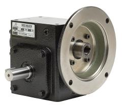
IronHorse heavy-duty worm gearbox, 15:1 ratio, 56C-Face input, left hand, 0.875in diameter output shaft, nominal 0.75hp at 1.0 SF, 554 lb-in mechanical output torque, 1-3/4in center distance, cast iron housing, tapped-base mount.
