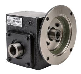
IronHorse heavy-duty worm gearbox, 15:1 ratio, 56C-Face input, hollow, 1in diameter output shaft, nominal 0.75hp at 1.0 SF, 554 lb-in mechanical output torque, 1-3/4in center distance, cast iron housing, tapped-base mount.
