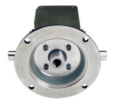
IronHorse heavy-duty worm gearbox, 15:1 ratio, 56C-Face input, dual, 0.875in diameter output shaft, nominal 0.75hp at 1.0 SF, 554 lb-in mechanical output torque, 1-3/4in center distance, cast iron housing, tapped-base mount.
