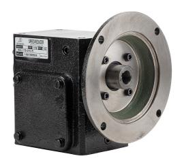
IronHorse heavy-duty worm gearbox, 10:1 ratio, 56C-Face input, right hand, 0.875in diameter output shaft, nominal 1hp at 1.0 SF, 515 lb-in mechanical output torque, 1-3/4in center distance, cast iron housing, tapped-base mount.
