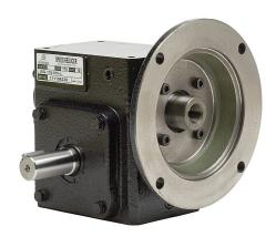
IronHorse heavy-duty worm gearbox, 10:1 ratio, 56C-Face input, left hand, 0.875in diameter output shaft, nominal 1hp at 1.0 SF, 515 lb-in mechanical output torque, 1-3/4in center distance, cast iron housing, tapped-base mount.
