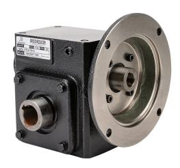
IronHorse heavy-duty worm gearbox, 10:1 ratio, 56C-Face input, hollow, 1in diameter output shaft, nominal 1hp at 1.0 SF, 515 lb-in mechanical output torque, 1-3/4in center distance, cast iron housing, tapped-base mount.
