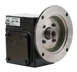
IronHorse heavy-duty worm gearbox, 5:1 ratio, 56C-Face input, right hand, 0.875in diameter output shaft, nominal 1.5hp at 1.0 SF, 499 lb-in mechanical output torque, 1-3/4in center distance, cast iron housing, tapped-base mount.
