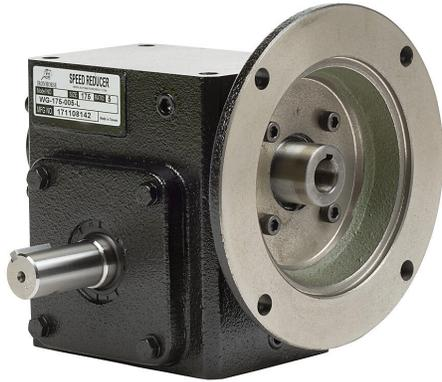
IronHorse heavy-duty worm gearbox, 5:1 ratio, 56C-Face input, left hand, 0.875in diameter output shaft, nominal 1.5hp at 1.0 SF, 499 lb-in mechanical output torque, 1-3/4in center distance, cast iron housing, tapped-base mount.
