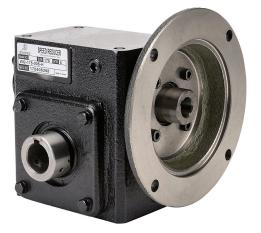
IronHorse heavy-duty worm gearbox, 5:1 ratio, 56C-Face input, hollow, 1in diameter output shaft, nominal 1.5hp at 1.0 SF, 499 lbin mechanical output torque, 1-3/4in center distance, cast iron housing, tapped-base mount.
