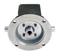
IronHorse heavy-duty worm gearbox, 5:1 ratio, 56C-Face input, dual, 0.875in diameter output shaft, nominal 1.5hp at 1.0 SF, 499 lb-in mechanical output torque, 1-3/4in center distance, cast iron housing, tapped-base mount.
