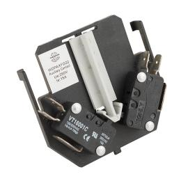
Worldwide Electric auxiliary contact, left or right side mount, (2) SPDT contact(s), 3A @ 120 VAC/0.5A @ 125 VDC. For use with WDP25 to WDP40 3-Pole contactors only. (2) Microswitches with 1/4in quick-connect terminals included.
