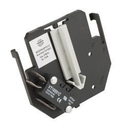
Worldwide Electric auxiliary contact, left or right side mount, (1) SPDT contact(s), 3A @ 120 VAC/0.5A @ 125 VDC. For use with WDP25 to WDP40 3-Pole contactors only. (1) Microswitch with 1/4in quick-connect terminals included.
