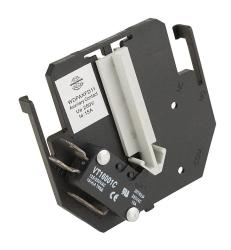
Worldwide Electric auxiliary contact, left or right side mount, (1) SPDT contact(s), 3A @ 120 VAC/0.5A @ 125 VDC. For use with WDP25 to WDP40 3-Pole contactors only. (1) Microswitch with 1/4in quick-connect terminals included.
