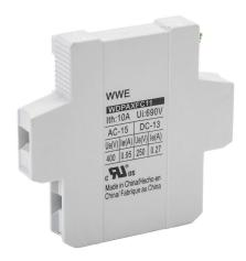
Worldwide Electric auxiliary contact, left or right side mount, (1) N.O./(1) N.C. contact(s), 3A @ 120 VAC/0.5A @ 125 VDC. For use with WDP25 to WDP60 3-Pole contactors only. Screw connection terminals included.
