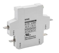
Worldwide Electric auxiliary contact, left or right side mount, (1) N.O./(1) N.C. contact(s), 3A @ 120 VAC/0.5A @ 125 VDC. For use with WDP25 to WDP60 3-Pole contactors only. 1/4in quick-connect terminals included.
