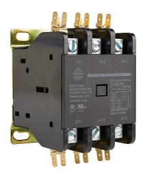
Worldwide Electric WDP series definite purpose contactor, 60A, (3) N.O. power poles, 230 VAC 50/60 Hz coil voltage. Box lugs with 1/4in quick-connect terminals included.
