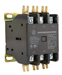
Worldwide Electric WDP series definite purpose contactor, 60A, (3) N.O. power poles, 120 VAC 50/60 Hz coil voltage. Box lugs with 1/4in quick-connect terminals included.
