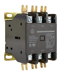
Worldwide Electric WDP series definite purpose contactor, 50A, (3) N.O. power poles, 230 VAC 50/60 Hz coil voltage. Box lugs with 1/4in quick-connect terminals included.
