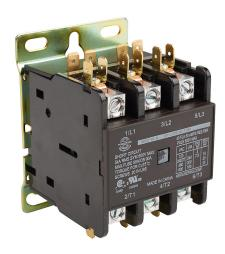
Worldwide Electric WDP series definite purpose contactor, 40A, (3) N.O. power poles, 480 VAC 50/60 Hz coil voltage. Box lugs with 1/4in quick-connect terminals included.
