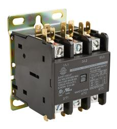
Worldwide Electric WDP series definite purpose contactor, 40A, (3) N.O. power poles, 230 VAC 50/60 Hz coil voltage. Box lugs with 1/4in quick-connect terminals included.
