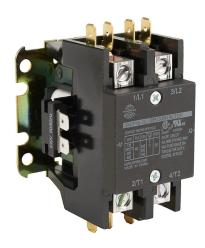
Worldwide Electric WDP series definite purpose contactor, 40A, (2) N.O. power poles, 230 VAC 50/60 Hz coil voltage. Box lugs with 1/4in quick-connect terminals included.
