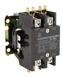
Worldwide Electric WDP series definite purpose contactor, 40A, (2) N.O. power poles, 120 VAC 50/60 Hz coil voltage. Box lugs with 1/4in quick-connect terminals included.
