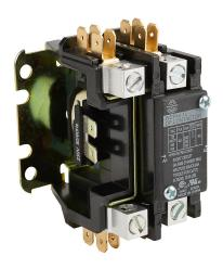
Worldwide Electric WDP series definite purpose contactor, 40A, (1) N.O. + shunt power poles, 230 VAC 50/60 Hz coil voltage. Box lugs with 1/4in quick-connect terminals included.
