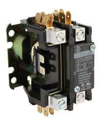
Worldwide Electric WDP series definite purpose contactor, 40A, (1) N.O. + shunt power poles, 120 VAC 50/60 Hz coil voltage. Box lugs with 1/4in quick-connect terminals included.
