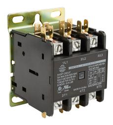
Worldwide Electric WDP series definite purpose contactor, 32A, (3) N.O. power poles, 480 VAC 50/60 Hz coil voltage. Box lugs with 1/4in quick-connect terminals included.
