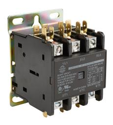
Worldwide Electric WDP series definite purpose contactor, 32A, (3) N.O. power poles, 230 VAC 50/60 Hz coil voltage. Box lugs with 1/4in quick-connect terminals included.
