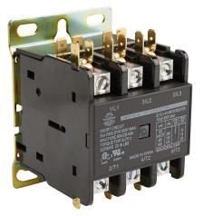
Worldwide Electric WDP series definite purpose contactor, 32A, (3) N.O. power poles, 120 VAC 50/60 Hz coil voltage. Box lugs with 1/4in quick-connect terminals included.
