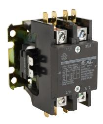
Worldwide Electric WDP series definite purpose contactor, 32A, (2) N.O. power poles, 24 VAC 50/60 Hz coil voltage. Box lugs with 1/4in quick-connect terminals included.
