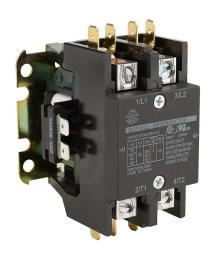
Worldwide Electric WDP series definite purpose contactor, 32A, (2) N.O. power poles, 230 VAC 50/60 Hz coil voltage. Box lugs with 1/4in quick-connect terminals included.
