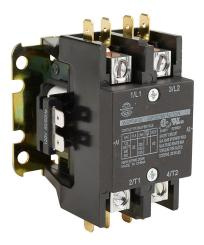
Worldwide Electric WDP series definite purpose contactor, 32A, (2) N.O. power poles, 120 VAC 50/60 Hz coil voltage. Box lugs with 1/4in quick-connect terminals included.
