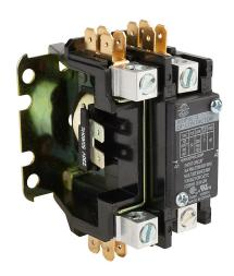
Worldwide Electric WDP series definite purpose contactor, 32A, (1) N.O. + shunt power poles, 230 VAC 50/60 Hz coil voltage. Box lugs with 1/4in quick-connect terminals included.
