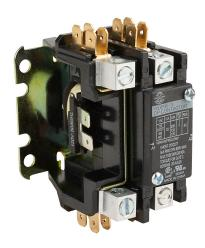
Worldwide Electric WDP series definite purpose contactor, 32A, (1) N.O. + shunt power poles, 120 VAC 50/60 Hz coil voltage. Box lugs with 1/4in quick-connect terminals included.
