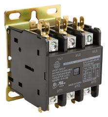
Worldwide Electric WDP series definite purpose contactor, 25A, (3) N.O. power poles, 230 VAC 50/60 Hz coil voltage. Box lugs with 1/4in quick-connect terminals included.
