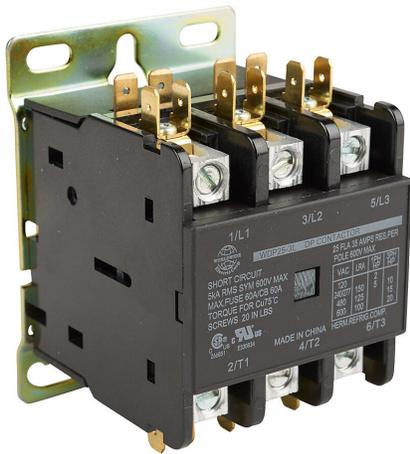
Worldwide Electric WDP series definite purpose contactor, 25A, (3) N.O. power poles, 120 VAC 50/60 Hz coil voltage. Box lugs with 1/4in quick-connect terminals included.
