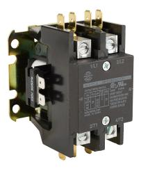
Worldwide Electric WDP series definite purpose contactor, 25A, (2) N.O. power poles, 230 VAC 50/60 Hz coil voltage. Box lugs with 1/4in quick-connect terminals included.
