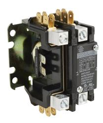
Worldwide Electric WDP series definite purpose contactor, 25A, (1) N.O. + shunt power poles, 230 VAC 50/60 Hz coil voltage. Box lugs with 1/4in quick-connect terminals included.
