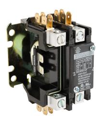
Worldwide Electric WDP series definite purpose contactor, 25A, (1) N.O. + shunt power poles, 120 VAC 50/60 Hz coil voltage. Box lugs with 1/4in quick-connect terminals included.
