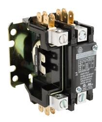
Worldwide Electric WDP series definite purpose contactor, 25A, (1) N.O. + shunt power poles, 120 VAC 50/60 Hz coil voltage. Box lugs with 1/4in quick-connect terminals included.
