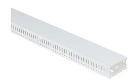
AchieVe WDN series open slot narrow finger wire duct, 3in width, 1.5in height, 6.5ft/2m length, white. Cover included.
