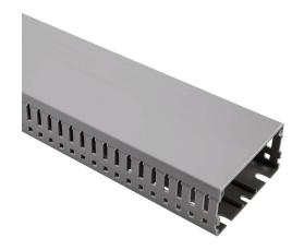
AchieVe WDN series open slot narrow finger wire duct, 3in width, 1.5in height, 6.5ft/2m length, gray. Cover included.
