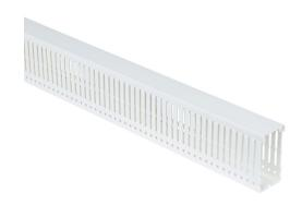
AchieVe WDN series open slot narrow finger wire duct, 1.5in width, 3in height, 6.5ft/2m length, white. Cover included.
