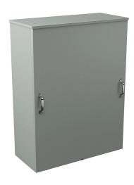
Wiegmann enclosure, NEMA 1/3R, 48 x 36 x 16in (HxWxD), wall mount, carbon steel, ANSI 61 gray, powder coat finish, screw cover with handles, padlock hasp and staple.
