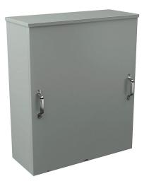
Wiegmann enclosure, NEMA 1/3R, 36 x 30 x 12in (HxWxD), wall mount, carbon steel, ANSI 61 gray, powder coat finish, screw cover with handles, padlock hasp and staple.
