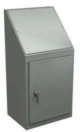
Wiegmann operator console, NEMA 12/13, 48 x 24 x 18in (HxWxD), freestanding, carbon steel, ANSI 61 gray, powder coat finish, single-door, 3-point keylocking handle.
