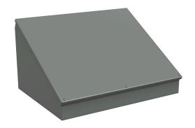
Wiegmann operator consolet, NEMA 12/13, 20 x 24 x 13in (HxWxD), desktop or pedestal mount, carbon steel, ANSI 61 gray, powder coat finish.
