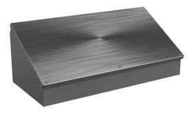
Wiegmann operator consolet, NEMA 4/4X/12/13,  $12 \times 24 \times 9$ in (HxWxD), desktop or pedestal mount, 304 stainless steel, No. 3 intermediate polished finish.
