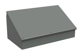
Wiegmann operator consolet, NEMA 12/13, 12 x 20 x 9in (HxWxD), desktop or pedestal mount, carbon steel, ANSI 61 gray, powder coat finish.
